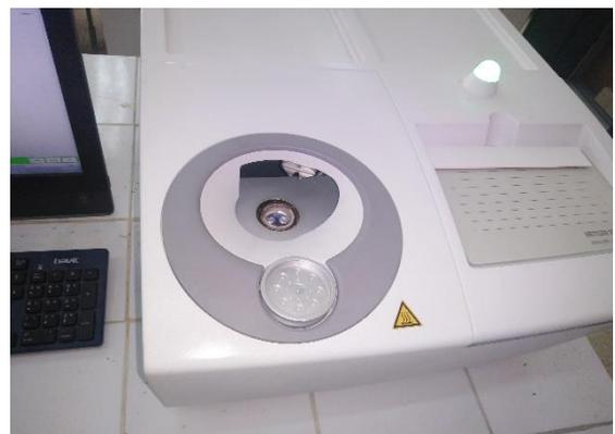
**Figure III.4** Machine de DSC model *METTLER TOLEDO DSC*.
