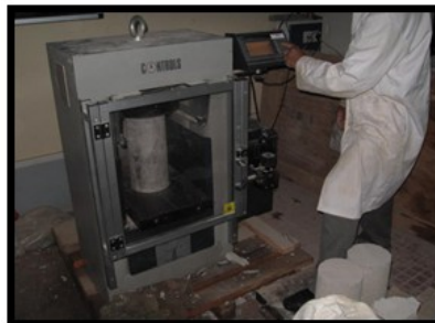
Figure II.12: Ecrasement des cylindres en compression.
