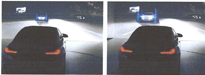
Figure 3.2: Car Tracking In RMW Cam - Used to exclude other cars from BMW car's Laser lights [37].
