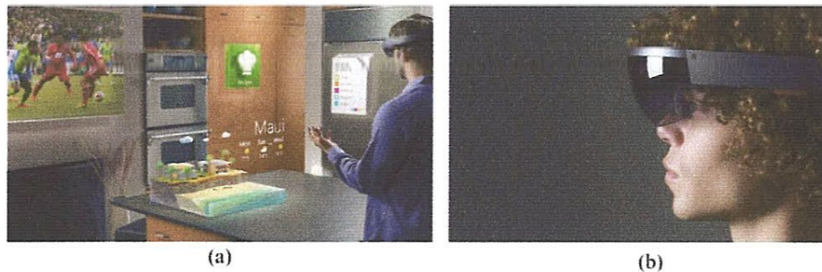
Figure 1.4: Microsoft HoloLens : (a) A new commercial mixed reality experience, of the real world and a virtual world combined using computer vision techniques of HoloLens, (b) Microsoft's new HoloLens, unveiled in January 21st, 2015[9].
