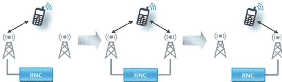
Figure I.13 : Exemple de soft Handover. [5]
