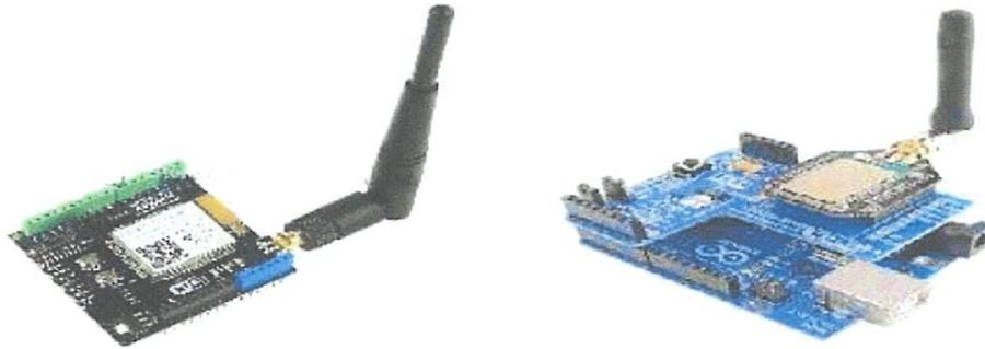
Figure II.8 : Module shield wifi
