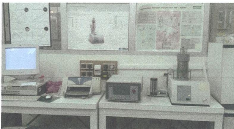
Figure 5.9 – La NETZSCH - STA 409 PC Luxx
