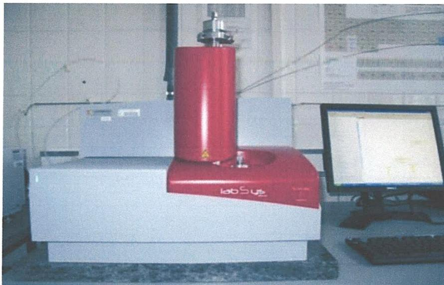
*Figure.III.4 : Appareil DSC de type LABSYS evo.*
