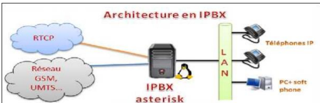
Figure II.7: Architecture de l'IPBX
