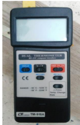
Figure II.12: Dual Channel Thermometer (RS-232 computer interface) model (TM-915A)
