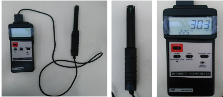
Figure II.10: Humidity/ Anemometer Meter – Lutron (AM-4205 A)
