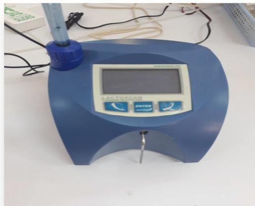
**Figure 6** : Lactoscan ULTRASONIC MILK ANALYSER.
