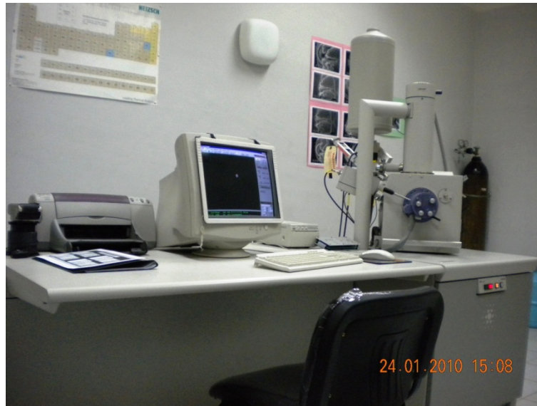
Figure II.10: Microscope MEB de type ESEM XL30.
