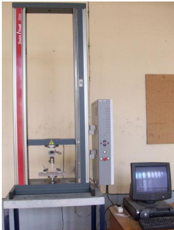
Figure II.18 : Machine universelle de type ZWICK ROELLE Z005
