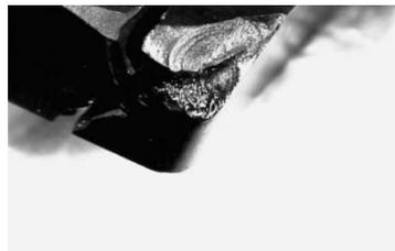
**Figure I.10** Rupture brutale du bec [LIU 02].
