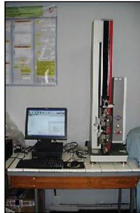
Figure II.21: Machine d'essai universelle Type Zwick 1120
