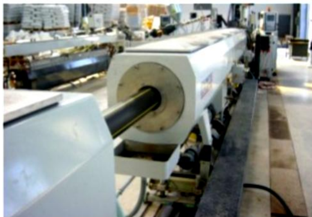
Figure II.8: Fabrication des tubes en PE
