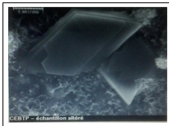
Photo III.2.6 : Cristal de chloroaluminate
