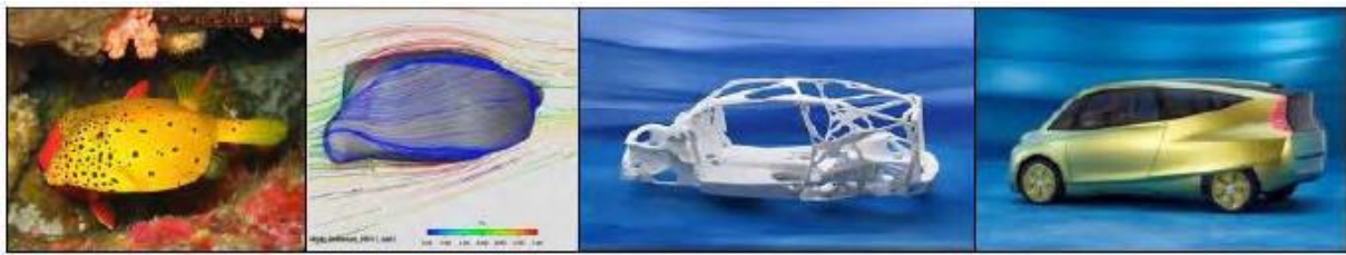
Fig 1.4: DaimlerCrysler bionic car inspired by the box fish and tree growth patterns. (Source: Pedersen Zari, M. 2007).
