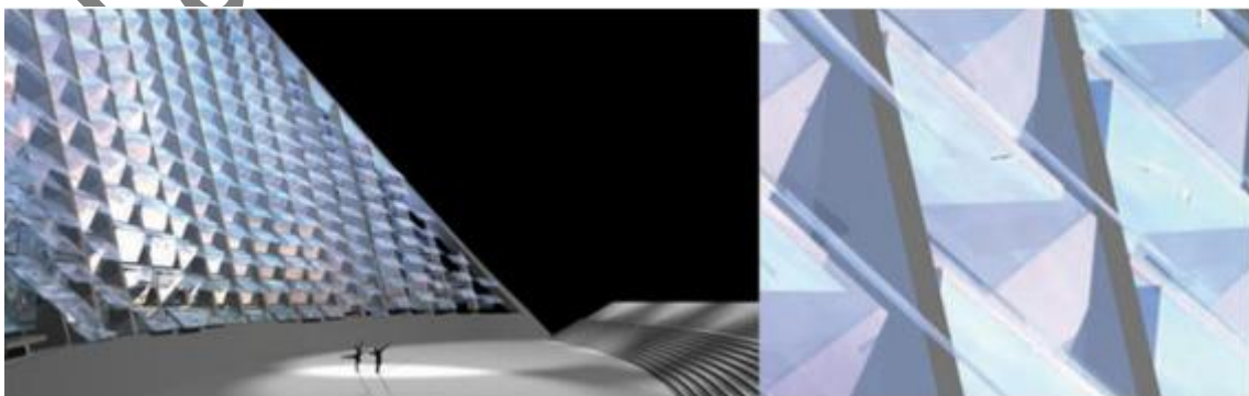
Fig 1.20 Las Palmas Water Theatre. Different wind flaps adjusting to the wind direction.
