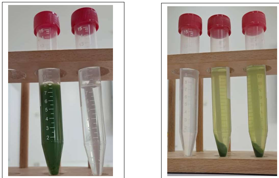
Fig 28: State of centrifuge tubes contain heterogenous mixture of parsley before and after separation by centrifugation
