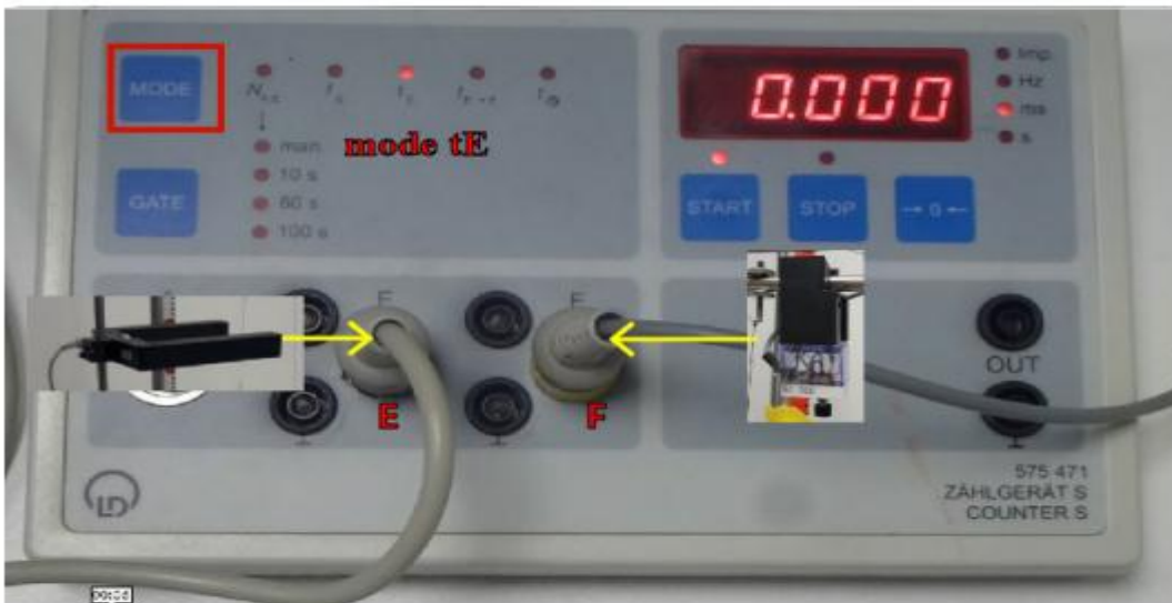
Figure 3: Measurement of time \Delta t to calculate the translation speed V , at the light barrier
