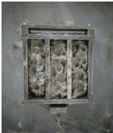
Figure II.22 : vibration des moules
