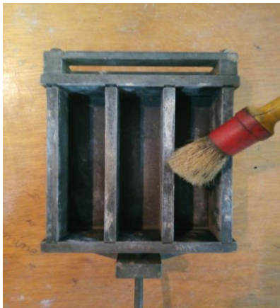
Figure II.21 : Lubrification des moules (4 x 4 x 16) cm 3
