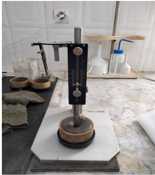
Figure II.15 : Essai de la consistance normale des ciments
