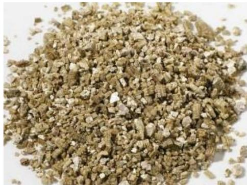
**Photo I.9:** Vermiculite expansée
