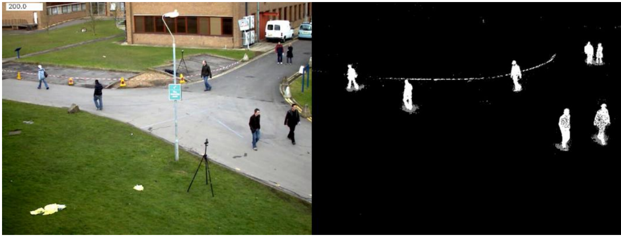
Figure II.4: Example of background subtraction [54].
