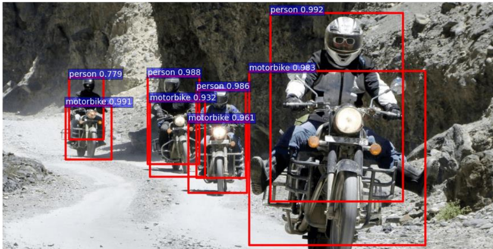
Figure II.2: Example of recognizing moving objects in an image [51].
