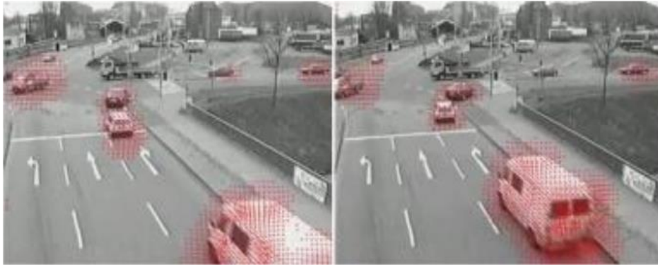
Figure II.3: Example of optical flow estimation [53].
