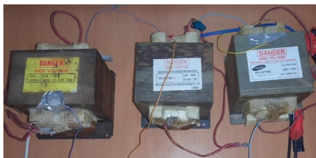
Figure III. 3: Three microwave transformers
