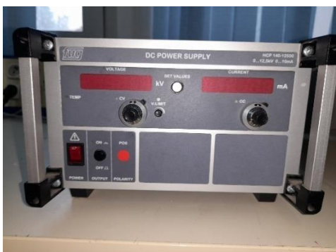
Figure III. 14: Positive High voltage source
