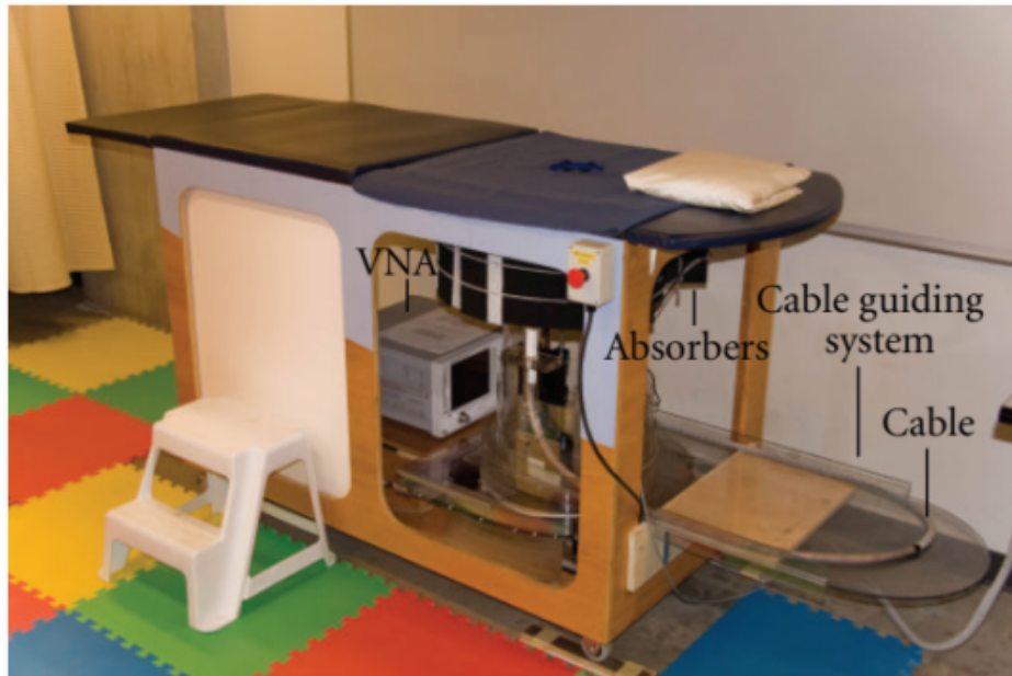
Figure 3.10: Prototype of the TSAR Radar-Based MI System for Breast Cancer Detection by Fear et al [135].
