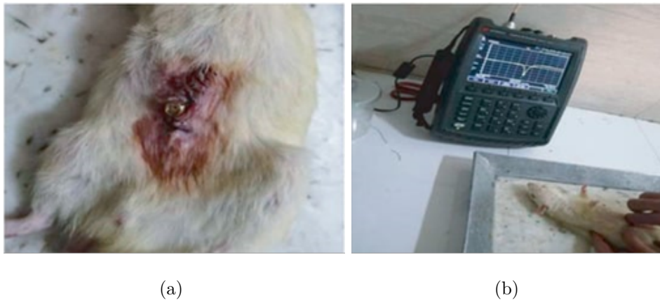
Figure 2.16: Continuous glucose monitoring using multi-layer implanted antenna sensor. (a) A rat with a sensor implanted; (b) the experimental setup [114].
