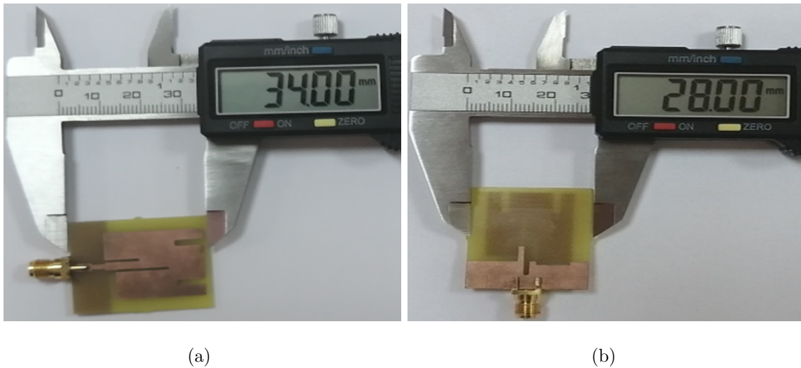
Figure 4.6: Manufactured prototype of the designed CPPMA : (a) front view, (b) back view.
