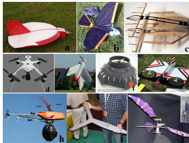
Figure 2.3: Different types of MAVs, (a) fixed wing, (b) flapping wing, (c) fixed/flapping-wing, (d) rotary wing, (e) VTOL, (f) ducted fan, (g) tilt-rotor, (h) helicopter, (i) unconventional, (j) ornicopter [10].
