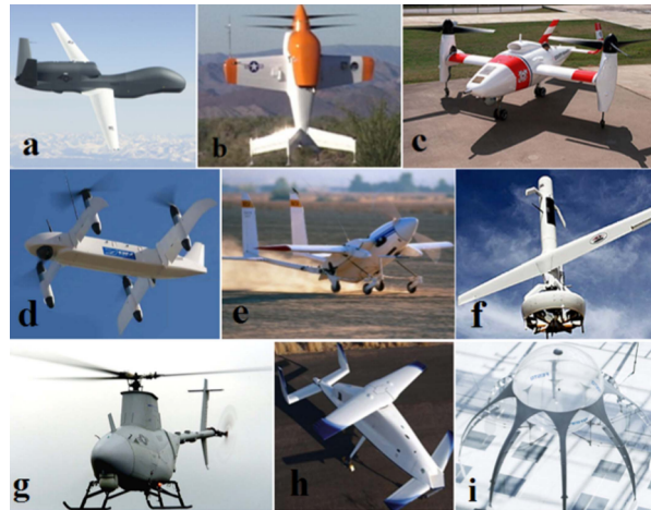
Figure 2.2: Different types of UAVs, (a) HTOL, (b) VTOL, (c) tilt-rotor UAV, (d) tilt-wing UAV, (e) tilt-body UAV, (f) ducted fan UAV, (g) helicopter, (h) heli-wing, and (i) unconventional UAV [10].
