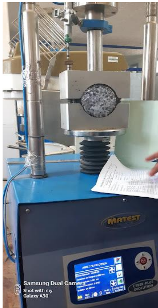
Figure 1.16. Automatic Marshall Stability Test Machine
