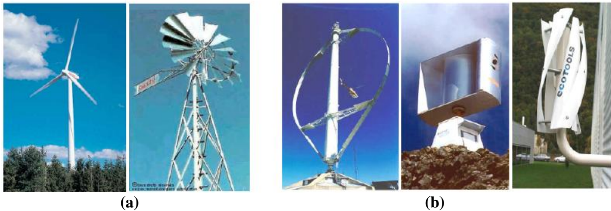
Figure (II.6) : Photos of main categories of wind turbines, (a) horizontal-axis wind turbine, (b) vertical-axis wind turbine [13].
