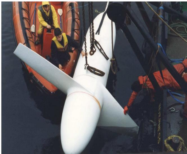
Figure (III.1) : World's first tidal turbine of IT Power Consulting Ltd [3].
