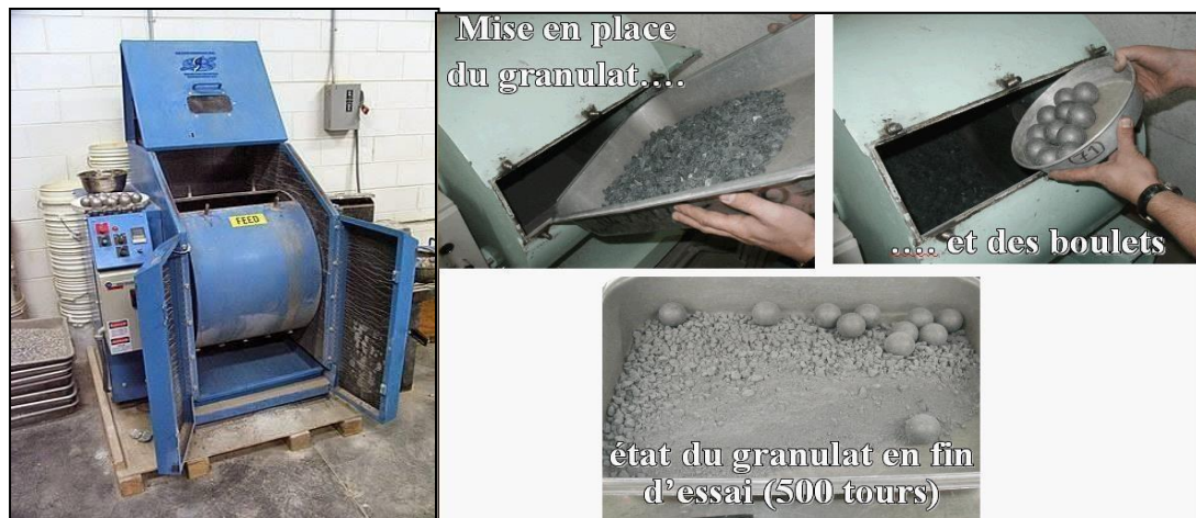
Figure II.8 : Essai Los Angeles.
