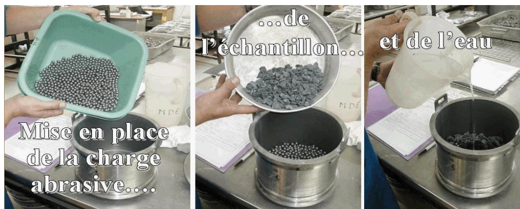
Figure II.9 : Essai Micro Deval.
