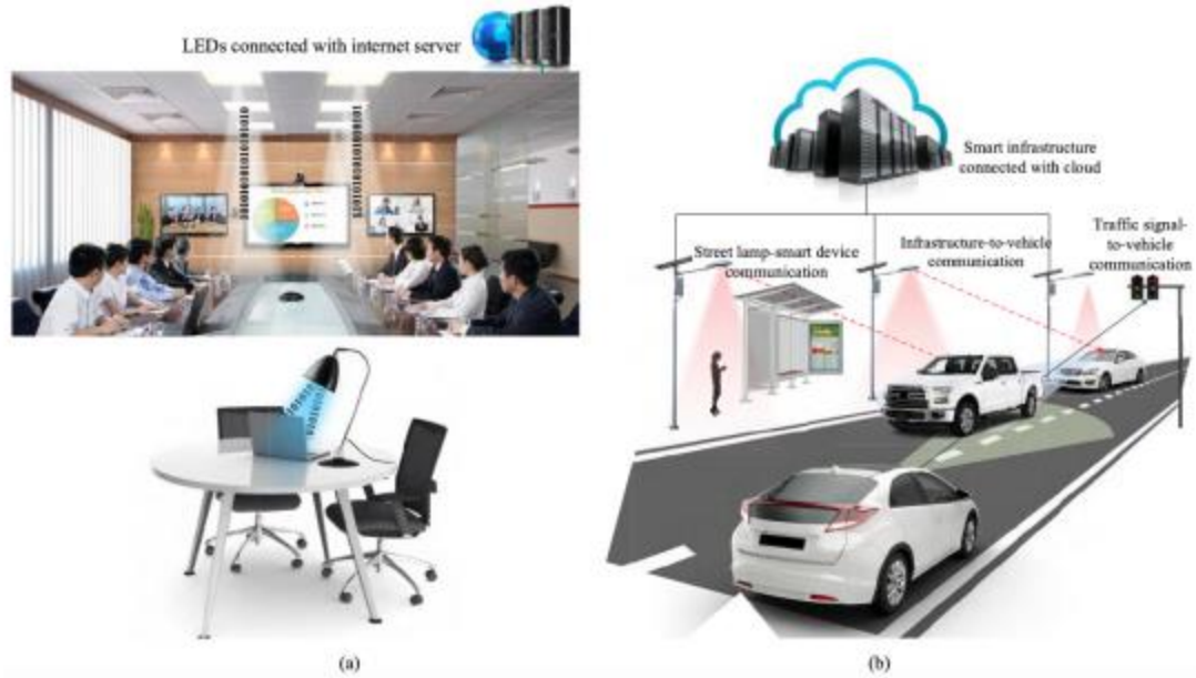
Fig I.20. Application Scenarios for VLC/LiFi; (a) Indoor Applications and (b) Outdoor Applications [35]
