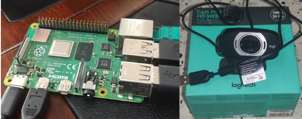
Fig.III.3: Our Raspberry pi + webcam
