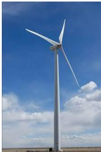
Figure 1.3 - Eolienne à axe horizontal, (The DOE 1.5 wind turbine at Site 4.0. Photo by Jeroen van Dam, National Renewable Energy Laboratory, https://www.nrel.gov/docs/fy15osti/63679.pdf )
