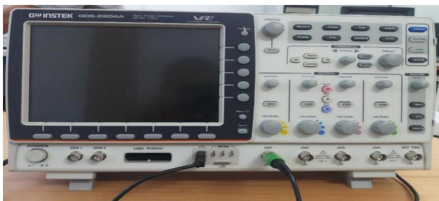
**Figure II.7:** Oscilloscope
