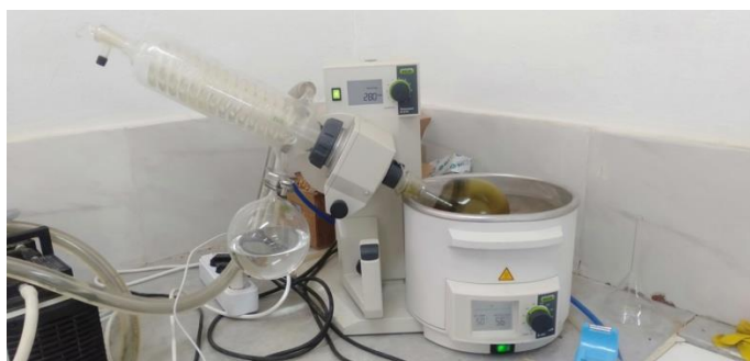
Figure 09: The separation of the solvent and pure oil by rota-evaporator (personal.2022).
