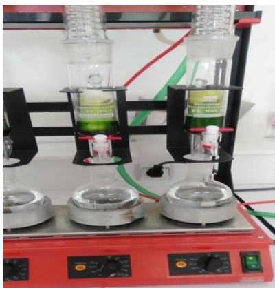
Figure 07: Soxhlet hydro-alcoholic extraction (personal, 2022).
