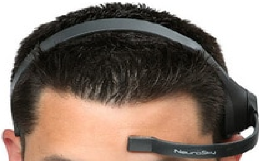
Figure IV.3: the positioning of EEG electrode on the forehead
