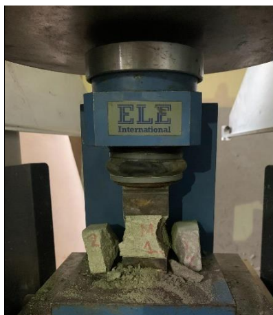
Figure III.8. Essai de compression.
