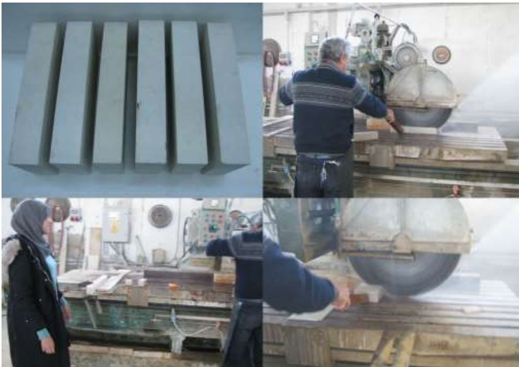
Fig. IV.6. Samples stone extracted from the Gaagaa quarry ( Source: The Author ).
