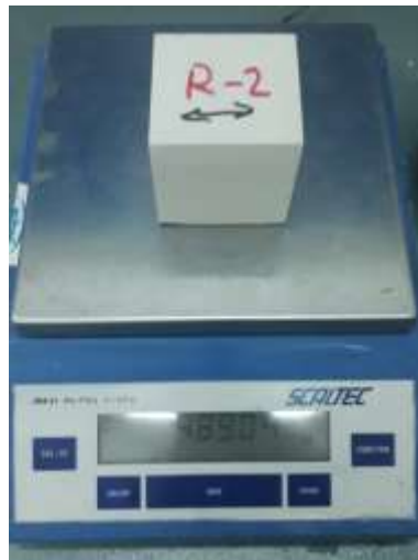
Fig. IV.10. Weighting the sample (Source: The Author).
