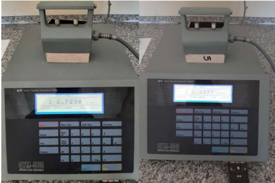
Fig. IV.7. Thermal properties test (Source: The Author).
