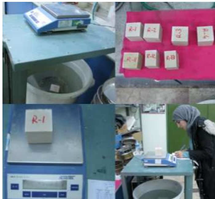
Fig. IV.8. Weighing of samples in Archimedean scales in water and saturated with water (Source: The Author).
