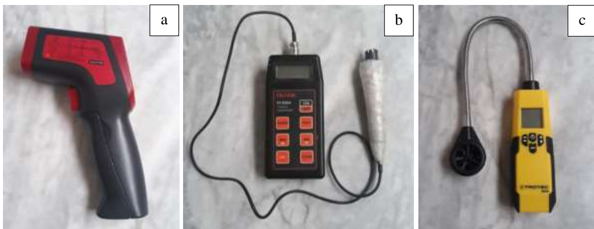
Fig. III.10. Measurement instruments; (a) Infrared thermometer. (b) Hygro-thermometer. (c) Thermal anemometer (Source: The Author).
