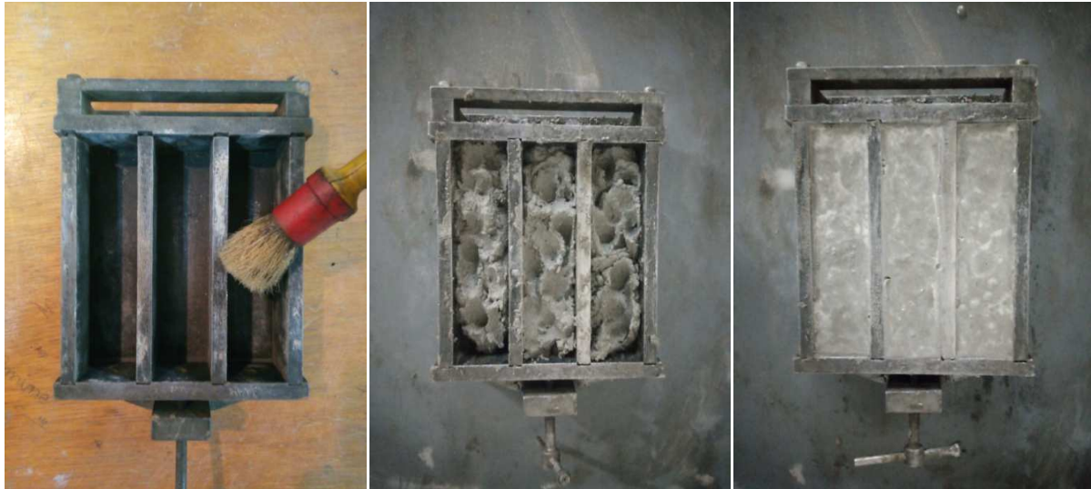
Figure II.23: Lubrification des moules (4 x 4 x 16)cm 3 .
