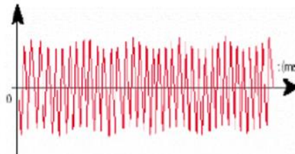
Figure (I.9) : Fluctuations de tension.
