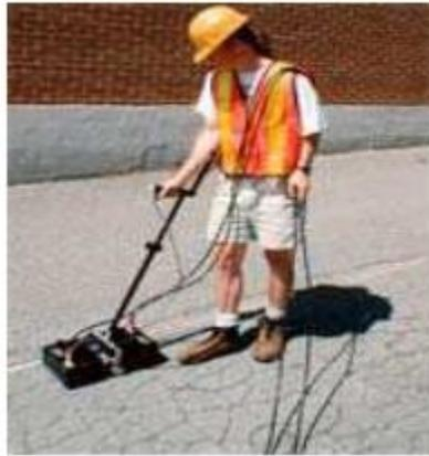
**Figure 1.15:** *Radar GPR pulse EKKO 1000.*
