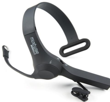
Figure 12 : Casque EEG NeuroSky Mindwave Mobile 2.
