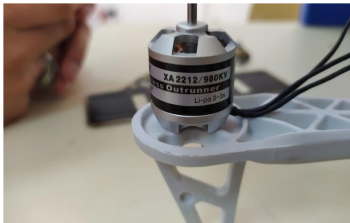
Figure III- 2: Moteur Brushless 980 KV.
