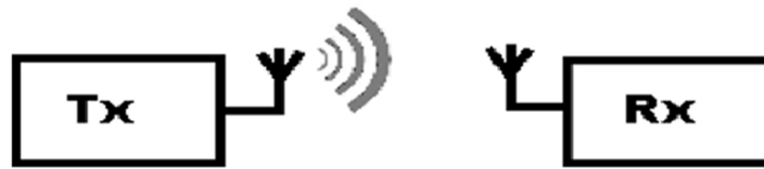
Figure II.1 SISO - Single Input Single Output
