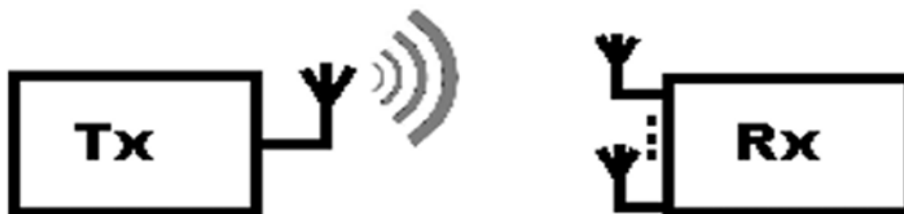
Figure II.2 SIMO - Single Input Multiple Output
