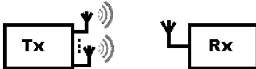
Figure II.3 MISO - Multiple Input Single Output
