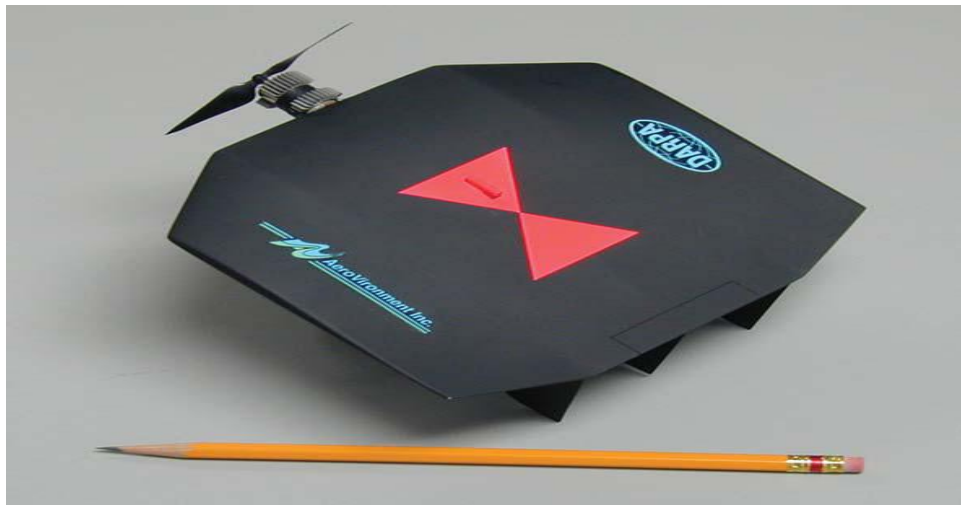
Figure (1-1): Micro-drone (black widow).
