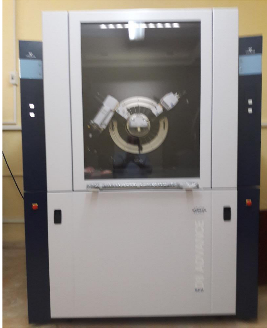
Figure II. 9: Diffractomètre des Rayons X «BRUKER D8 ADVANCE: LSPN Guelma»
