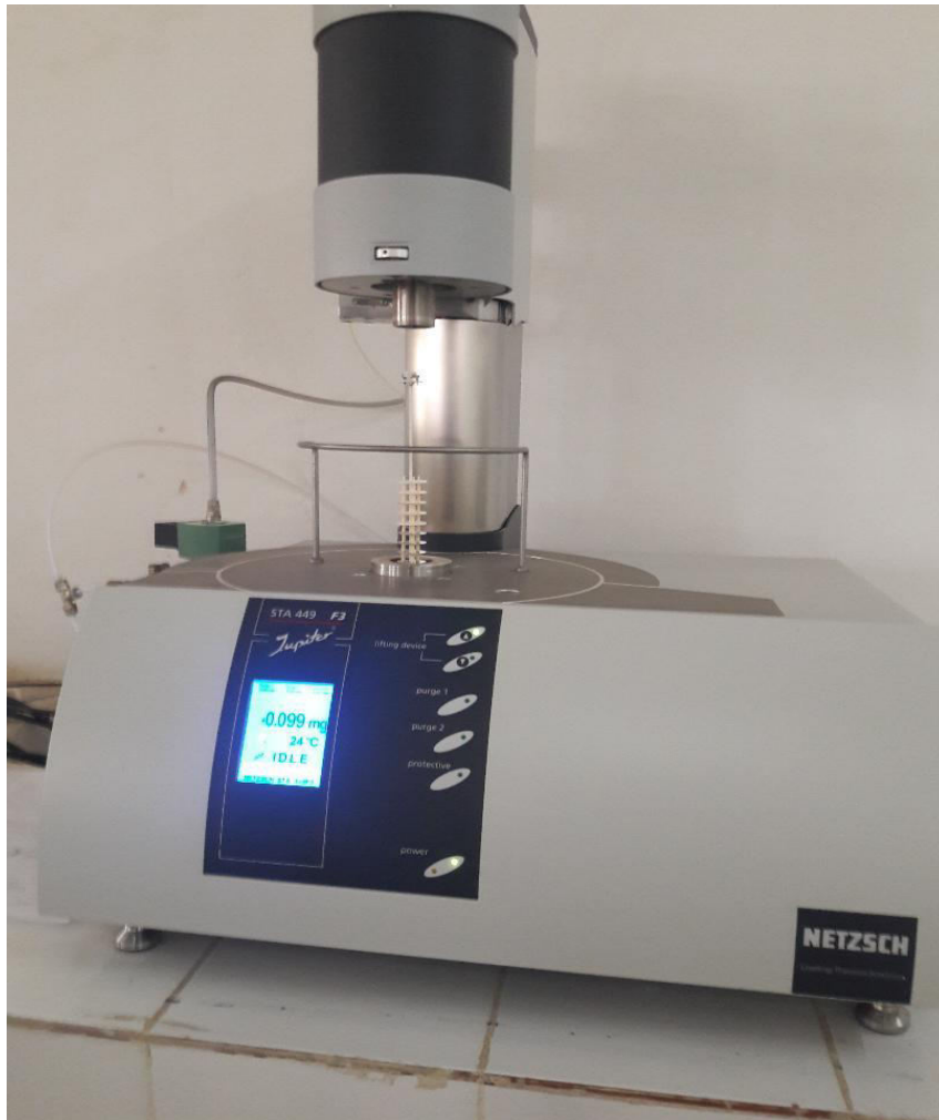
Figure II. 11: Appareil DSC type NETZSCH STA 449 F3 Jupiter: LSPN Guelma.
