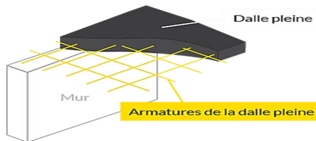
Figure I.6 Plancher dalle pleine.
