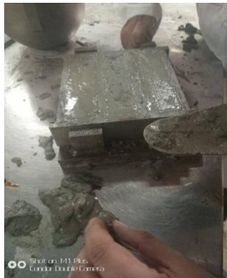
Figure III.17: Dernière vibration et rasage.
