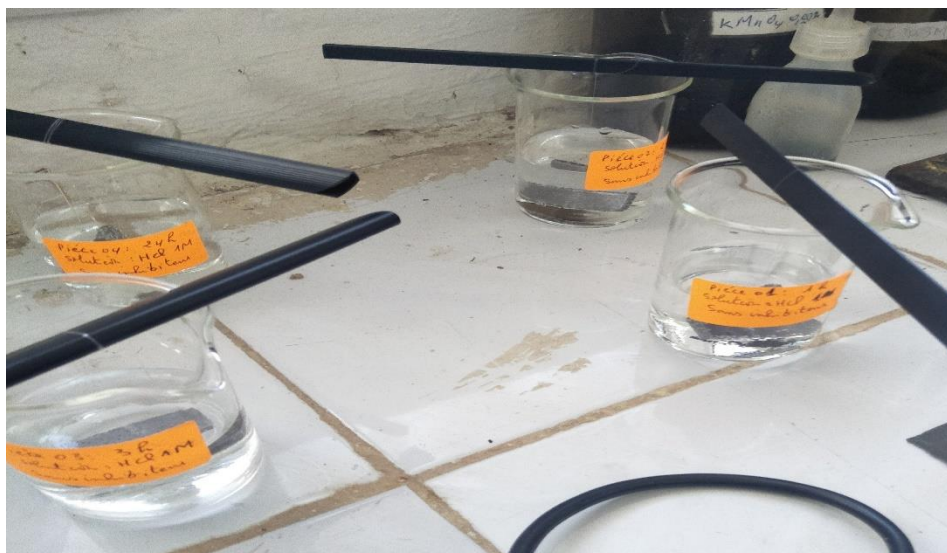
Figure III.11: L'essai de la corrosion
