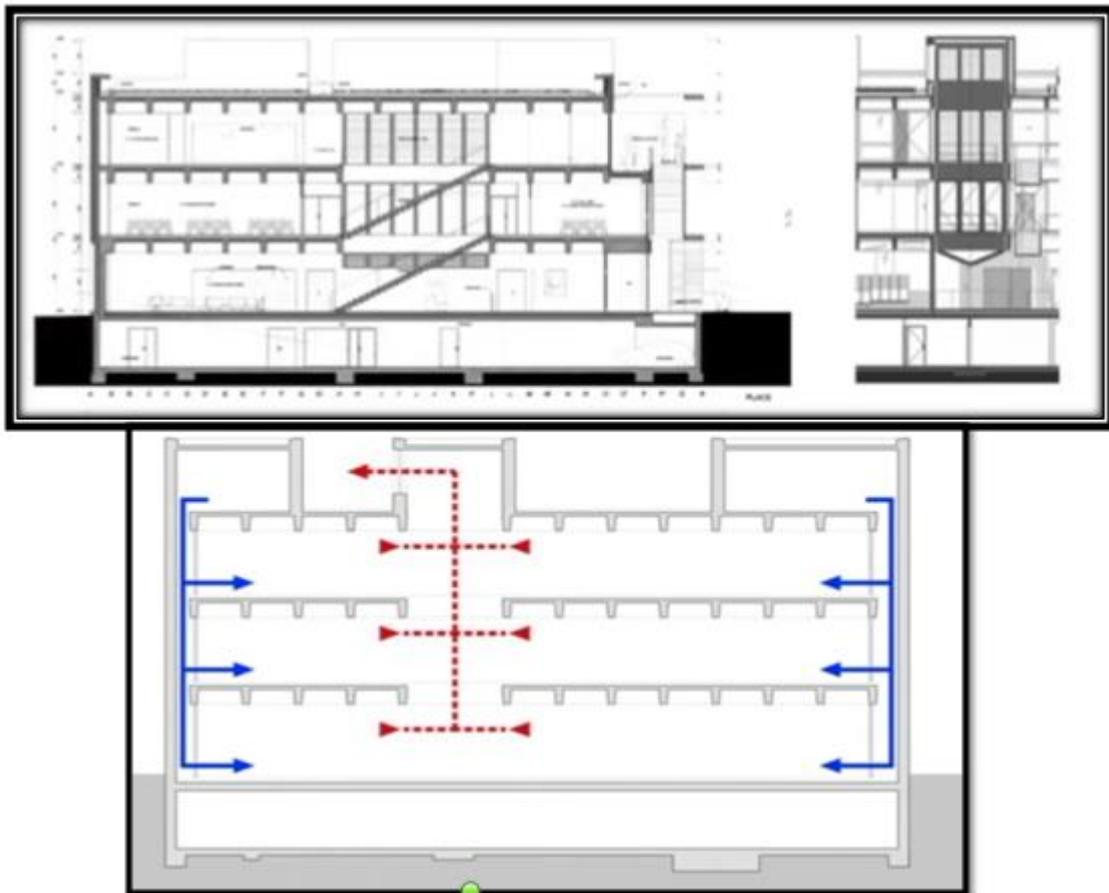
Figure 62: Principe de climatisation (source : <https://www.dailymotion.com/video/x6an0nk> )
