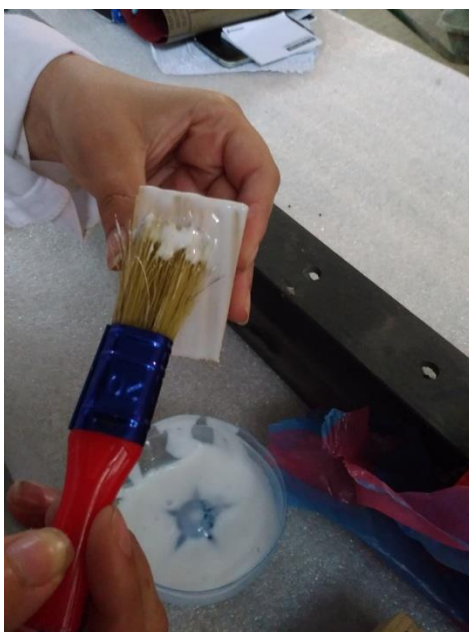
Figure I. 4: Application de la colle.
