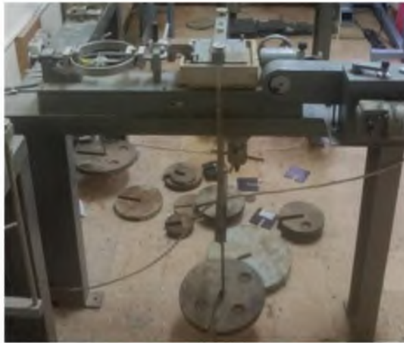
Figure 3.7 Application des charges verticales
