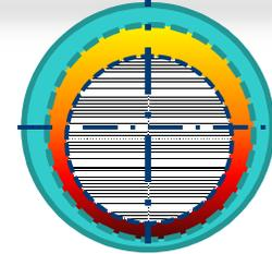
Foil bearing: Static and dynamic deformations
