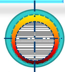
$$\frac{1}{R^2} \frac{\partial}{\partial \theta} \left[ \frac{G(h,l)}{12\mu} p \frac{\partial p}{\partial \theta} \right] + \frac{\partial}{\partial z} \left[ \frac{G(h,l)}{12\mu} p \frac{\partial p}{\partial z} \right] = \frac{\omega}{2} \frac{\partial (ph)}{\partial \theta} + \frac{\partial (ph)}{\partial t}$$
