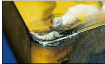
*Figure I-11: Oxydation*
