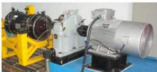
(a) Photo of the aero-engine rotor tester
